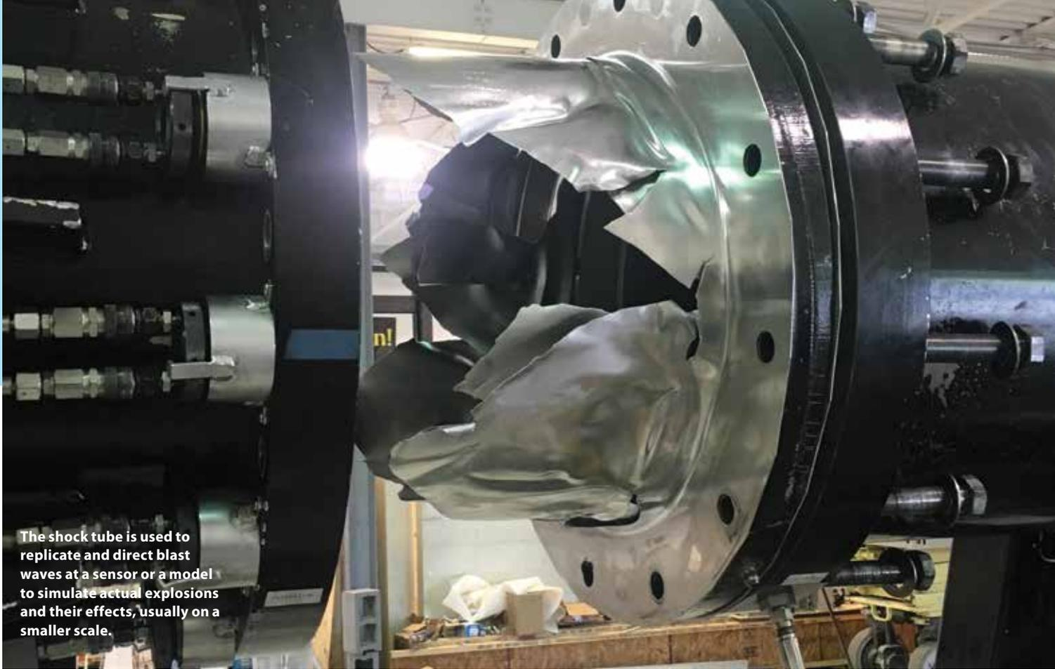
The shock tube is used to replicate and direct blast waves at a sensor or a model to simulate actual explosions and their effects, usually on a smaller scale.
