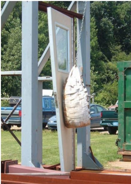
**This lightweight, flexible FRP door was tested for structural strength by repeatedly slamming it with a bag filled with 215 pounds of sand. The distance was increased incrementally until it reached a force of 750 ft-lb.**
