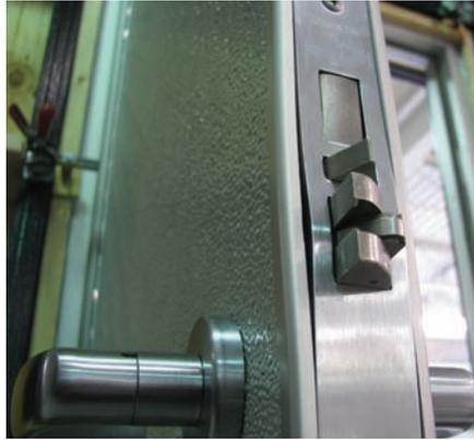
**This door was tested to the ASTM F 1642 protocol for blast resistance protection. When subjected to force in the 5.5 to 6.5 psi range, the door was slightly damaged, as seen in the bend of the aluminum at the fastener, but remained operational.**
